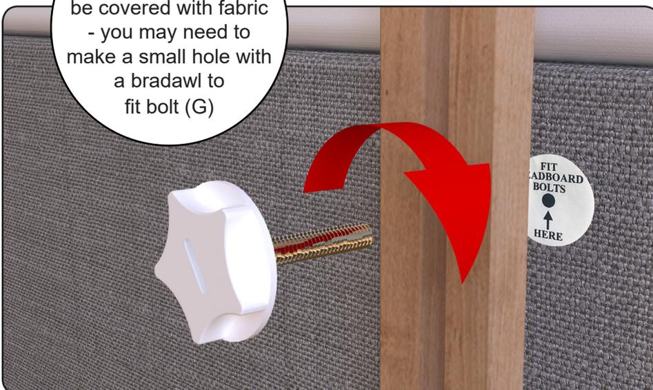
Fit headboard to bed using 4x bolts (G). These can be tightened by hand. Check your headboard is at preferred height and level before fully tightening.
